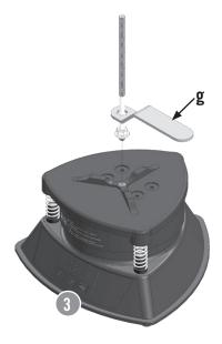
**6.** The Lid is held in place with the second Washer and Wing Nut.
